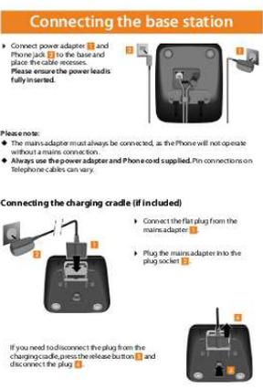
Connect power adapter (1) and Phone jack (2) to the base and place the cable across. Please ensure the power leads fully inserted.
