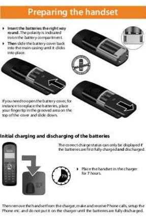
Insert the batteries the right way round. The polarity is indicated inside the battery compartment.
