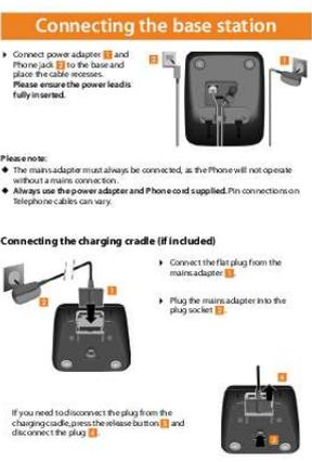
Connect power adapter (1) and Phone jack (2) to the base and plug the cable excess.
