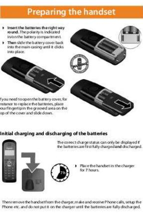
Insert the batteries the right way round. The polarity is indicated in the battery compartment.
