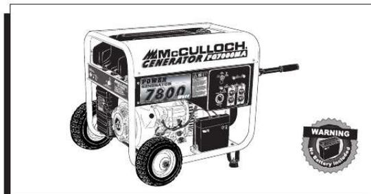
This generator is not equipped with park arrester which is required by U.S. forest service and the state of California.
