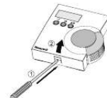
Fig. 1. DWM disassembly (T7560A,B)
