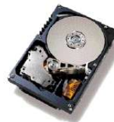
IBM Ultrastar 73LZX 3.5-inch 73.4 GB high-performance disk drive
