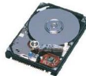
Travelstar 6GT 2.5-inch 6.4 GB 125mm disk drive
