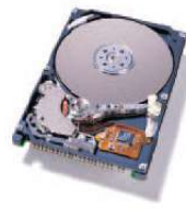
Travelstar 3GN 2.5-inch 3.2 GB ultra-low-profile disk drive
